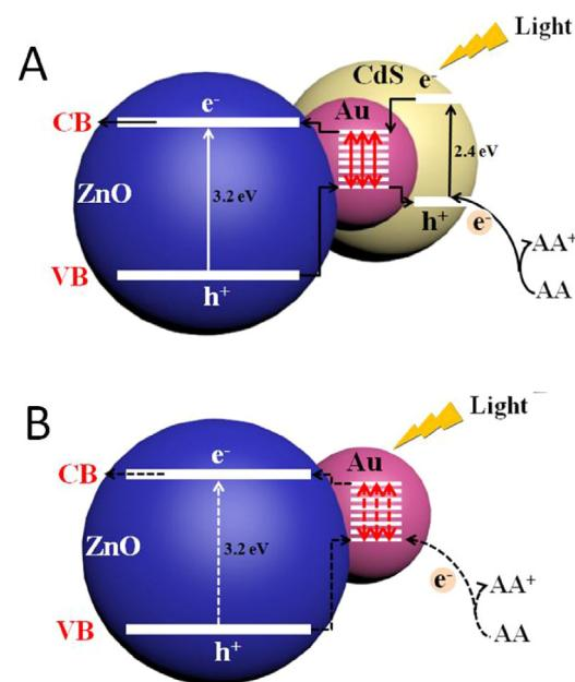
**Scheme 1.** Schematic of the charge-carrier transfer process in (A) the ZnO-Au@CdS microsphere and (B) ZnO-Au microsphere.
