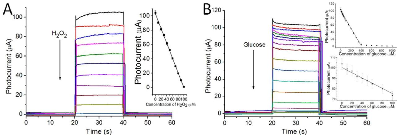
**Fig. 4.** Photocurrent response of the biosensor for the detection of different concentrations of (A) H<sub>2</sub>O<sub>2</sub> from 0 μM to 100 μM and (B) glucose from 0 μM to 1000 μM. The inset figures show the calibration curve with error bars with the standard deviation of three replicate determinations.
