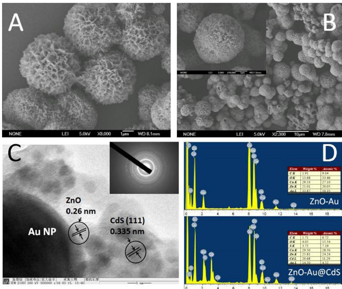
**Fig. 1.** SEM images of (A)ZnO, (B)ZnO-Au and the magnified ZnO-Au (inset), (C)HRTEM image of ZnO-Au@CdS and the corresponding SAED image (inset), and (D)EDS spectra of ZnO-Au and ZnO-Au@CdS and the corresponding elements contents.
