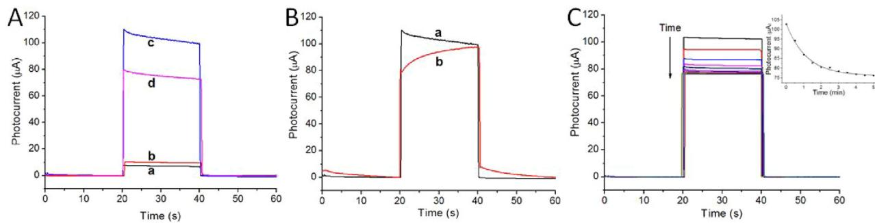
**Fig. 3.** (A) Photocurrent responses of the (a) ITO/GO/ZnO, (b) ITO/GO/ZnO-Au, (c) ITO/GO/ZnO-Au@CdS and (d) ITO/GO/ZnO-Au@CdS after bioetching. (B) Photocurrent responses of the (a) ITO/GO/ZnO-Au@CdS, (b) ITO/GO/ZnO@CdS. (C) The effect of bioetching time using 20 μM of H<sub>2</sub>O<sub>2</sub>.
