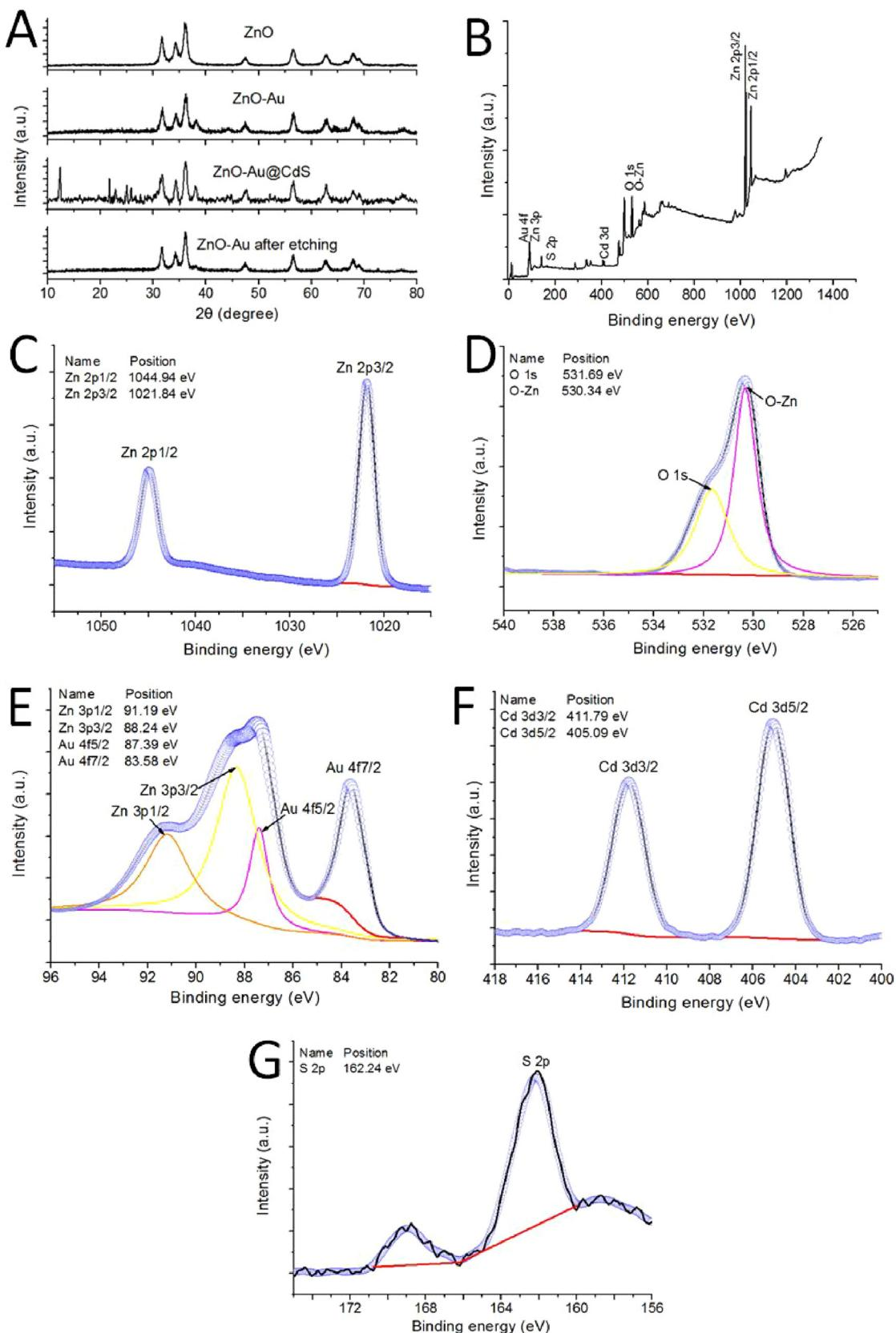
**Fig. 2.** (A) XRD of ZnO, ZnO-Au, ZnO-Au@CdS and ZnO-Au@CdS after bioetching. (B) Survey XPS spectrum of ZnO-Au@CdS, and (C-G) the high-resolution element spectrum.
