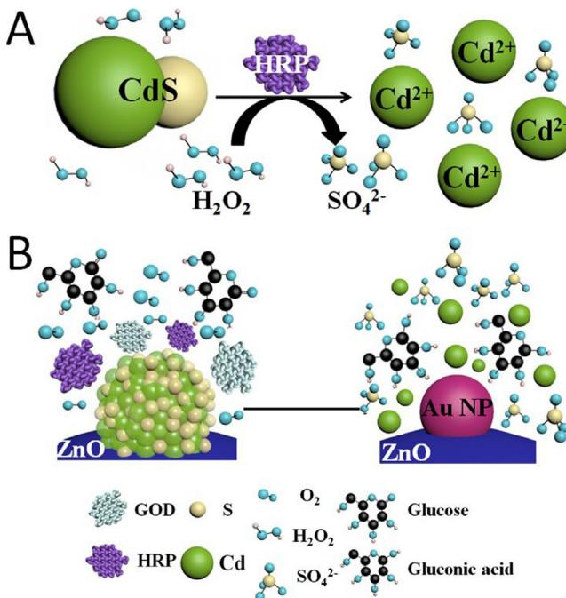
**Scheme 2.** Schematic illustration of (A) enzymatic bioetching of CdS NPs and (B) enzymatic bioetching process of the ZnO-Au@CdS biosensor.
